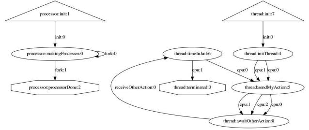
This is the diagram of the final **prisonerd2024.stm** showing all states and transitions. The goal of any player (thread within a process) is to minimize its time spent in the **timeInJail** state. Our simulation records that time for us to analyze. There are four strategies enumerated in **processor.action**, which my handout code places into each thread's **mystrategy** variable. Here are the strategies.
