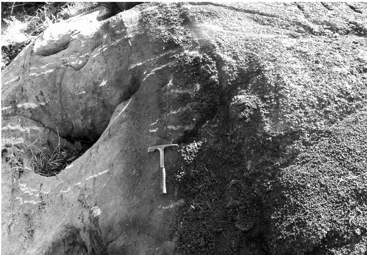
FIG. 5. Hammer rests on contact between granular magnetite ore on the right and sparsely mineralized marble from a deposit in the Franklin group. This style of mineralization is characteristic of most marble-hosted deposits in the New Jersey Highlands.
