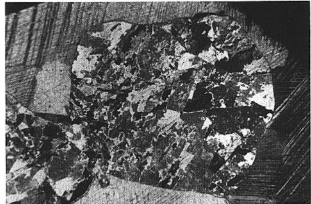
FIG. 7. Photomicrograph showing willemite pseudomorphous after tephroite within a few centimeters of a willemite-lined fracture. Field of view is about 0.5 mm, crossed polars.
